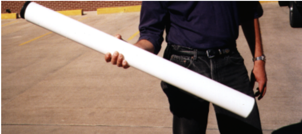
Figure 3B. Special equipment used for sampling water, bed sediment, and tissue at wetlands. Polytetrafluorethylene bed coring pipe.
